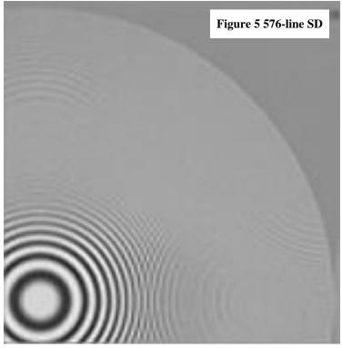
recommend using this camera in SD mode, because of the level of these spatial aliases. However, it is significantly better than the Z1 in this respect.
