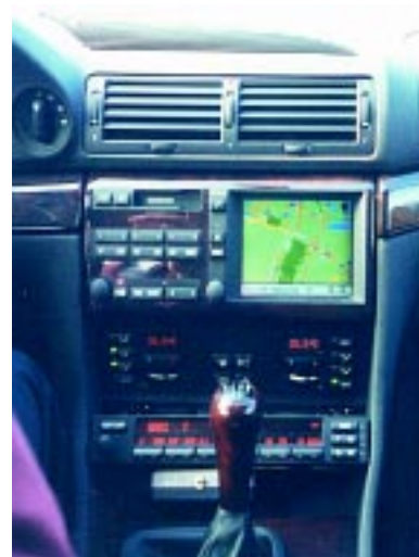
◀ Figure 5 An integrated car system – the Volvo RTI navigation system, using a two-tuner approach which separates the RDS-TMC facility from normal radio listening. (Source: Volvo)
