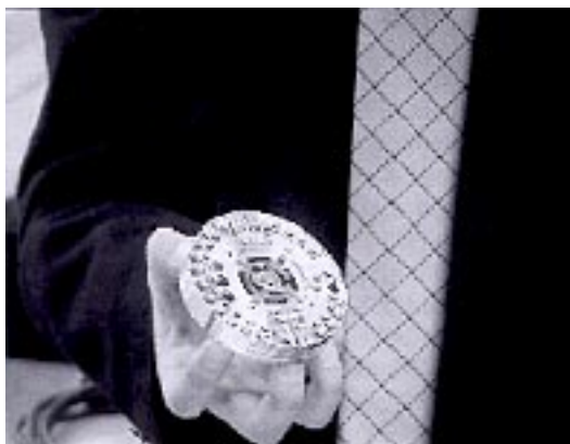
Figure 3 The scanner assembly from the Sony Betacam SX machine.
