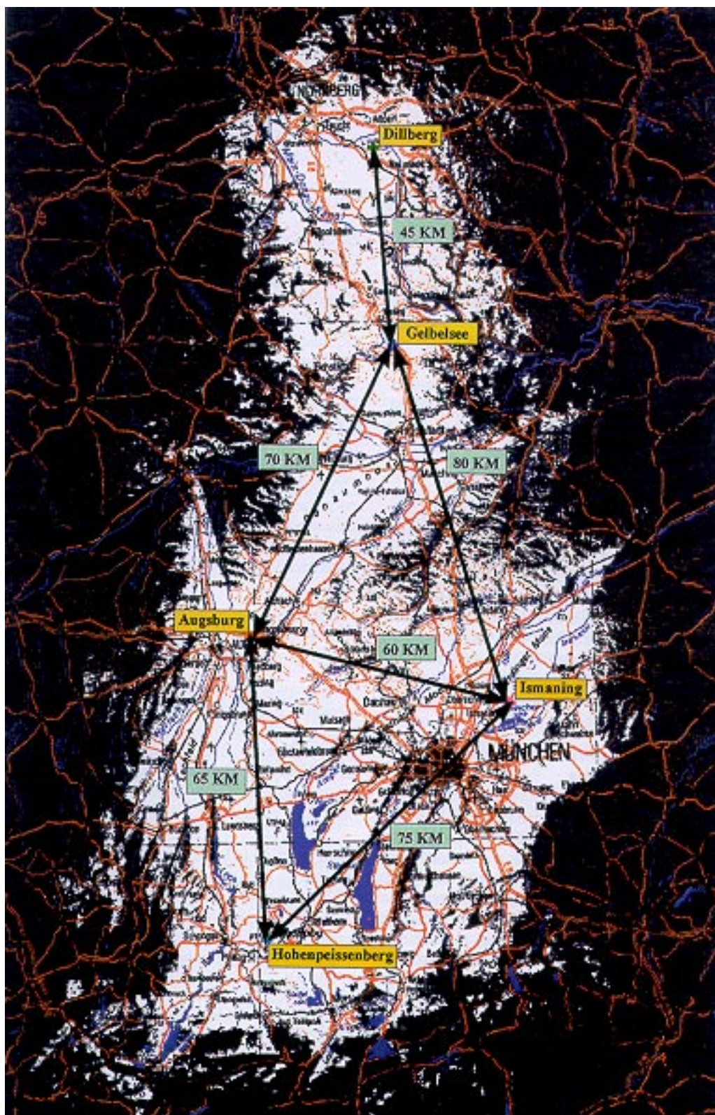
Fig. 2 Predicted coverage of the DAB SFN on channel 12. Addition of signals with power sum method; minimum wanted field-strength = 52 dB \mu V/m.
