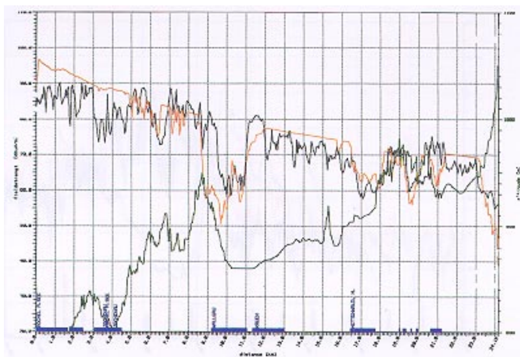
Fig. 21 Comparison of predicted and calculated field-strength. Route with reflected signals from surrounding mountains. (GEG DAB model, single transmitter)
