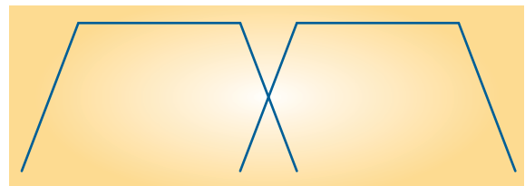
Figure 16 A variable-sized linear weighting matrix is used for overlapped block motion compensation to reduce block artefacts
