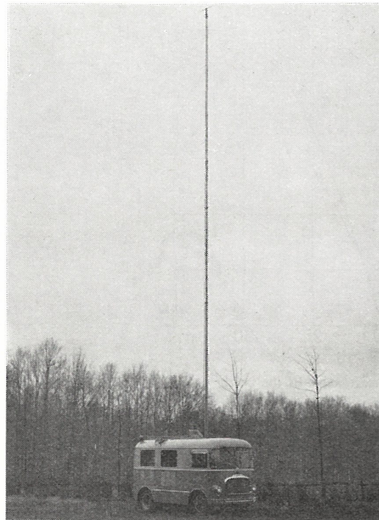
Fig. 6. — VHF/UHF field-strength measuring vehicle used by the RAI. The OM type "Tigrotto" 4-wheel-drive chassis carries a body built to Scall of Torino. The "Barberi" hydraulic mast can raise the aerial to a height of 23 m above the ground; its fully-retracted height is 2.5 m. The height of the aerial is indicated within \pm 1 cm by the device for running out the coaxial feeder.
