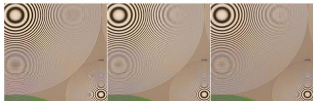
Figure 8 Zone plate, softening with ISO setting, 400, 1600, 6400
