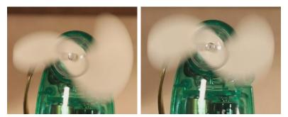
Figure 13 Rolling shutter effect, HD and 4K
