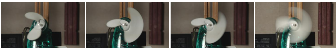
Figure 11 Motion distortion, e,f,g: 1/1000 shutter 1080i/25
