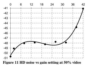
possible reasons for the unconventional shape in Fig. 9. Nevertheless, the noise level of -48dB is held up to 32dB gain, which is the equivalent of ISO 6400.
