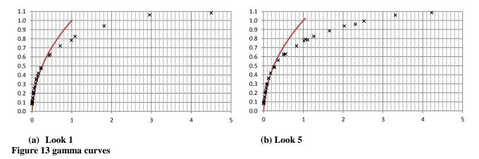
For sensitivity calculations, more multiple exposures were used to find the aperture setting at which the peak white patch reached 100%, when illuminated at 2000 lux. The camera was set to ISO800 (13.5dB gain) and Look1, 1/25 second exposure. The signal levels are not clipped at 100% video level and it was simple to find an exposure which reached exactly 100%, at between F/6.7 and F/7.3. So the sensitivity must be about F/5 at
