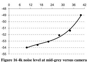
Figure 16 4k noise level at mid-grey versus camera gain in dB
