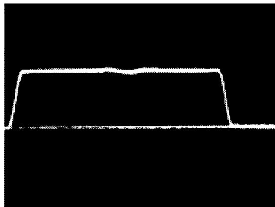
Fig 5 - Pulse display for correctly co-sited samples but with a small relative delay of about 10 ns
