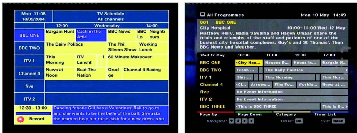
Figure 2 Screenshots of two EPGs for the same morning, taken from two makes of UK DTT set-top boxes
