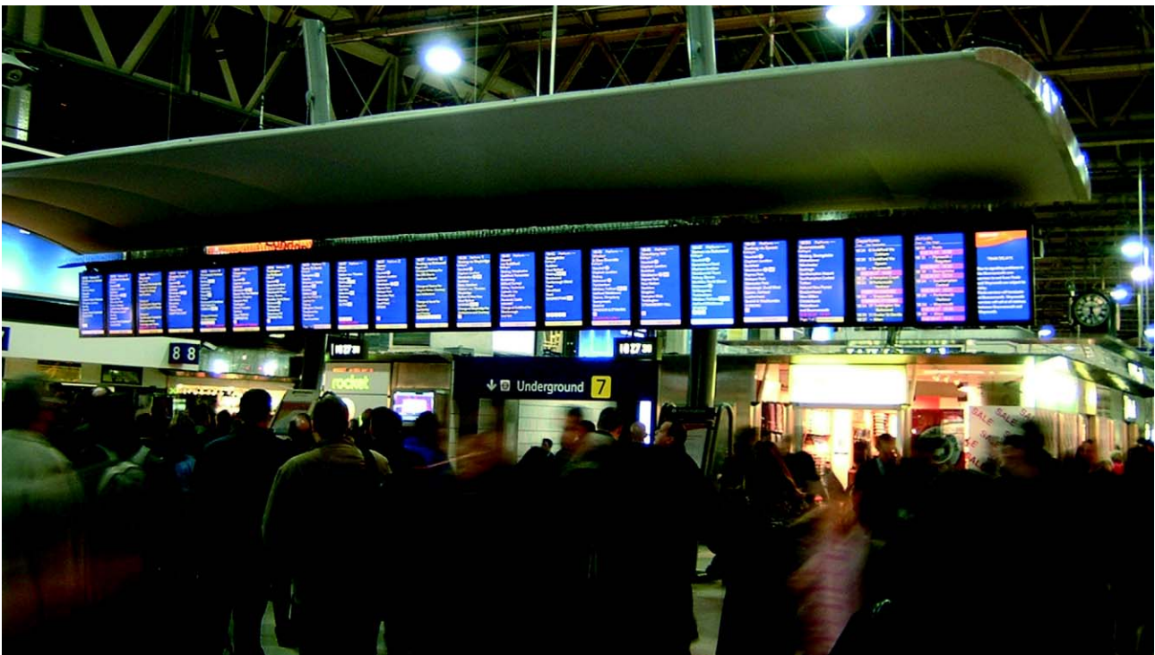
PDPs used as data displays in a major UK railway station. This photo indicates the brightness/contrast problem, which has had to be cured by placing ever larger canopies above the displays to block light coming in from the glass roof above, during daylight hours.
