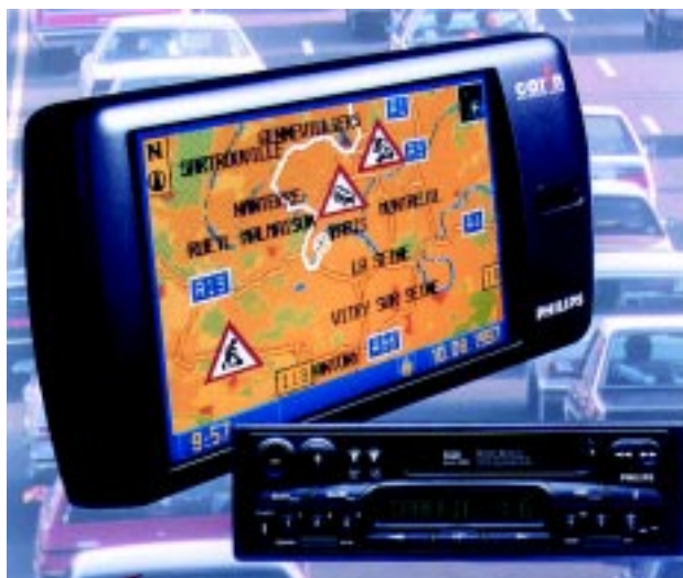
◀ Figure 5 An integrated car system – the Volvo RTI navigation system, using a two-tuner approach which separates the RDS-TMC facility from normal radio listening. (Source: Volvo)
