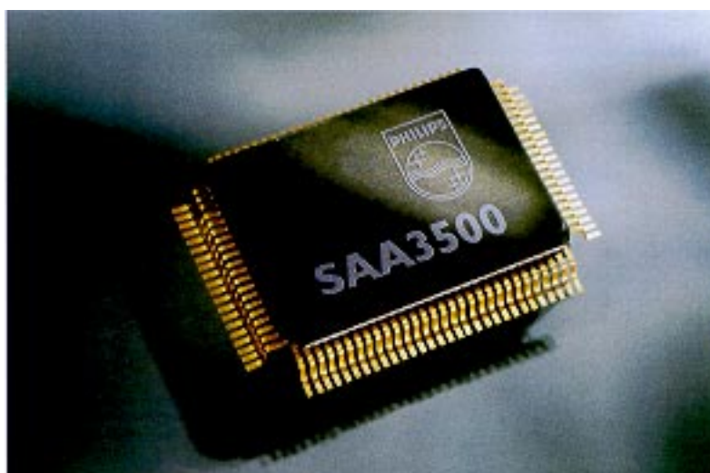
Figure 13 Preview of the SAA3500 DAB channel-decoder ASIC.
