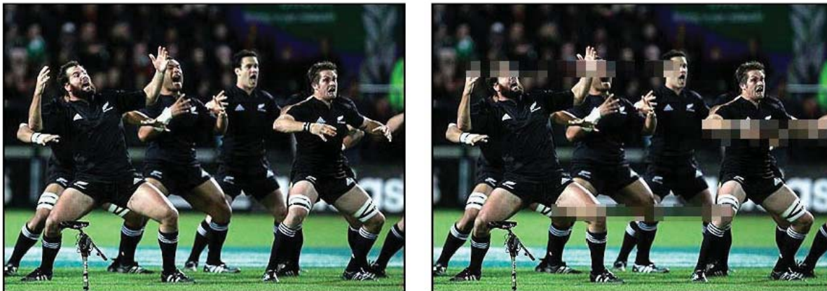
Figure 5 Same network impairment – but a very different impact on the viewer (Credit: Stefan Winkler, Symmetricom)
