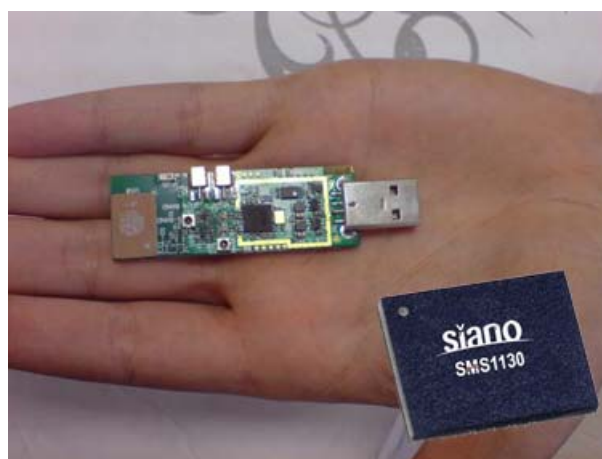
Figure 2 SMS1130 – multiple spectrum bands, multiple TV formats, single-chip, two-way DVB-T Diversity
