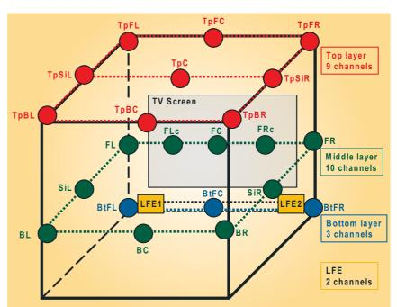
Figure 2 22.2 multichannel sound system
