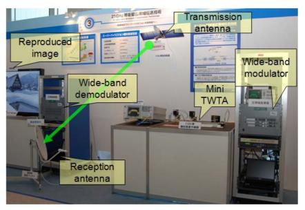
Figure 5 21-GHz-band indoor transmission experiment at open house in May 2007
