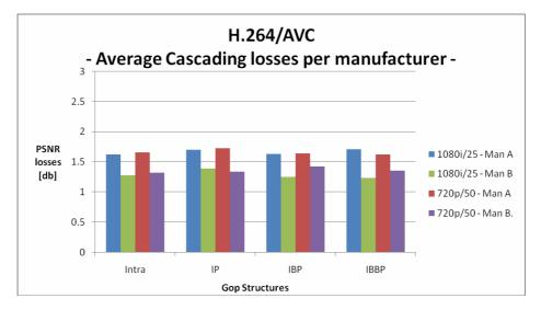
Figure 6: H.264/AVC average cascading losses per manufacturer
