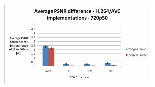
Figure 5: H.264/AVC Implementation differences with 720p/50 coding.
