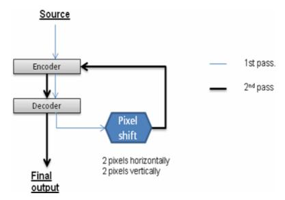
Figure 1: Simulation of a typical Contribution Link
