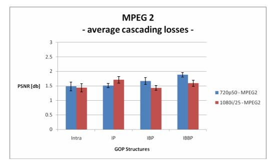
Figure 12: MPEG-2 average cascading losses
