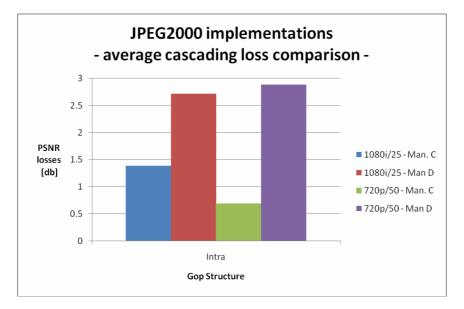
Figure 9: JPEG2000 average cascading losses
