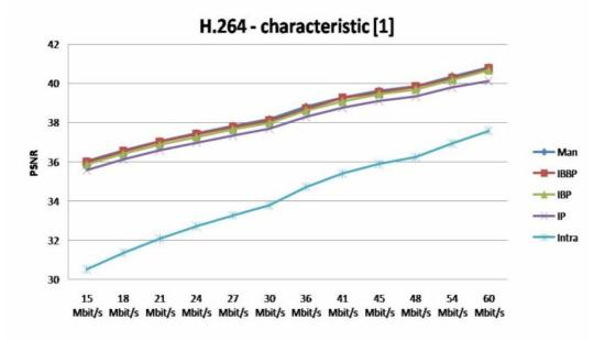
Figure 7: H.264/AVC system (1) characteristics
