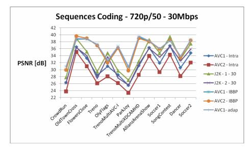
Figure 14: PSNR comparison of sequences. All systems encoded at 30 Mbit/s
