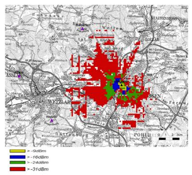
Figure E6: Regions potentially affected by cross-modulation
