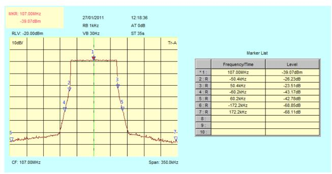
Figure G8: Recorded spectrum of DRM+ signal
