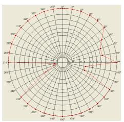
Figure C2: Radiation patterns of the new DRM+ transmitter
