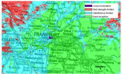
Figure C8: Cross-modulation within FM service area Pfaffenberg 88.4 MHz
