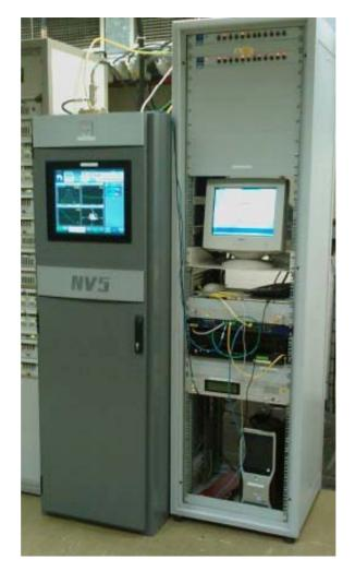
Figure G7: The DRM+ transmitter (left) and content server, modulator and monitoring receiver (right)
