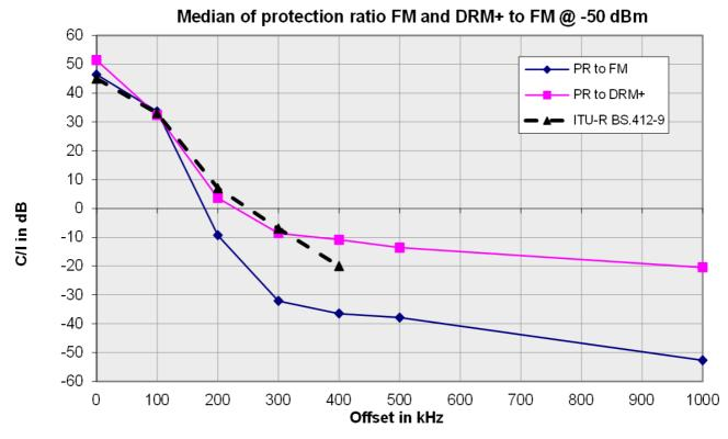
Figure F4: Median protection ratios for analogue and digital interferer (hifi tuners)
