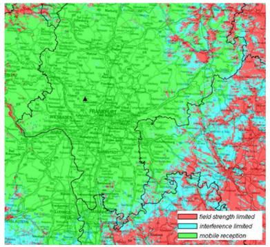
Figure D3: DRM+ mobile reception (4-QAM 1/3)
