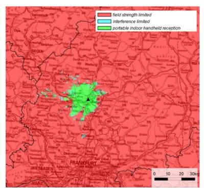
Figure E5: DRM+ portable indoor handheld reception (4-QAM 1/3)
