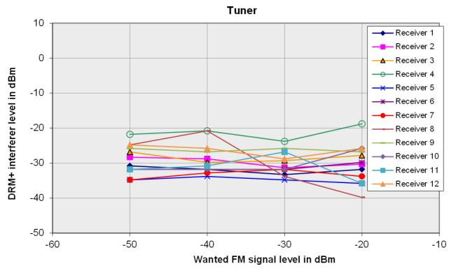
Figure F8: Allowable level of digital interfering signal vs. wanted FM signal level (hifi tuners)
