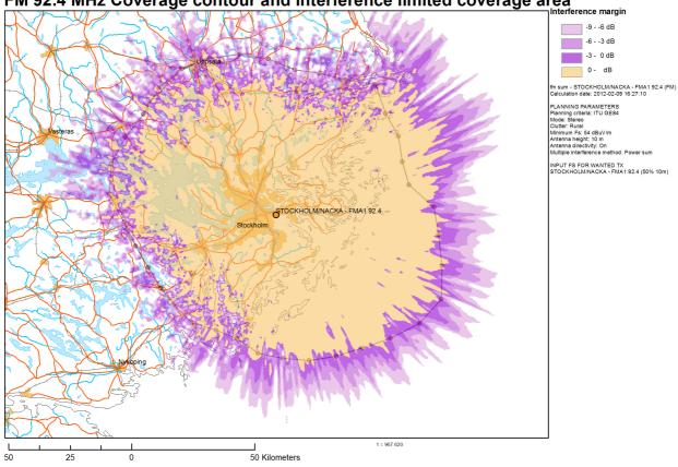
FM 92.4 MHz Coverage contour and interference limited coverage area
