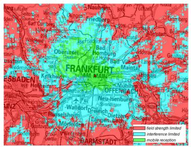
Figure C4: DRM+ mobile reception (4-QAM 1/3)
