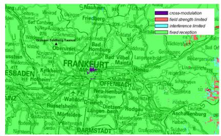
Figure C11: Cross-modulation within FM service area Grosser Feldberg 89.3 MHz
