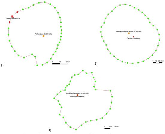
Figure C3: DRM+ transmitter and FM interference contours
