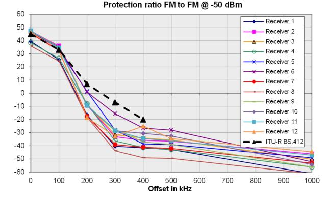
Figure F2: Measured protection ratios for FM interfered by FM; 12 hifi tuners
