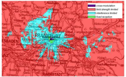
Figure C9: Cross-modulation within FM service area FfM Funkhaus 87.9 MHz
