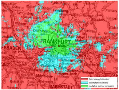
Figure C5: DRM+ portable indoor reception (4-QAM 1/3)
