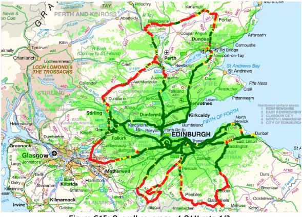
Figure G15: Overall coverage, 4-QAM rate 1/3.
