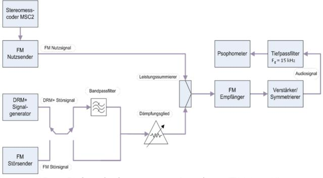
Figure F1: Setup for the measurement (in analogy to ITU-R Rec.641) of protection ratios for FM interfered with OFDM
