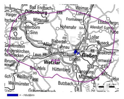
Figure E9: Interference contour of FM transmitter Wetzlar 90.5 MHz
