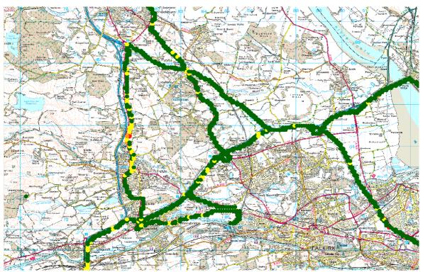
Figure G29: Falkirk to Stirling coverage, 4-QAM, rate 1/3
