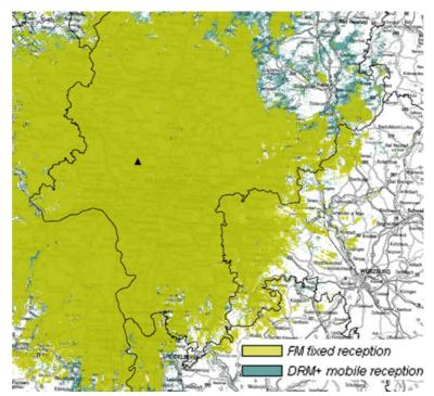
Figure D6: DRM+ mobile (4-QAM 1/3) versus FM fixed reception
