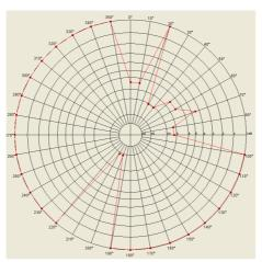
Figure E2: Radiation patterns of the new DRM+ transmitter Giessen 93.7 MHz
