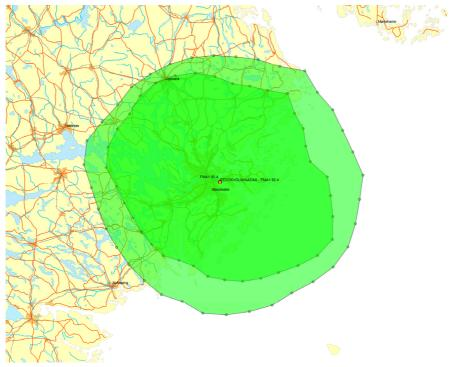
Figure B1: Noise and interference limited coverage for the FM transmitter at Stockholm/Nacka at 92.4 MHz.
