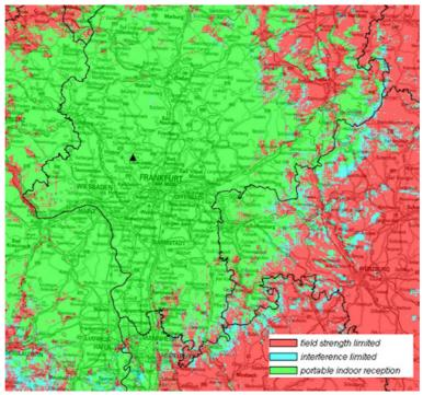
Figure D4: DRM+ portable indoor reception (4-QAM 1/3)
