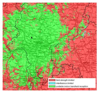
Figure D5: DRM+ portable indoor handheld reception (4-QAM 1/3)
