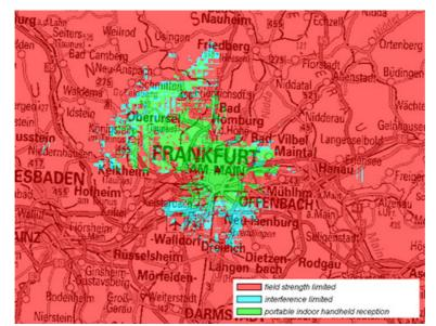
Figure C6: DRM+ portable indoor handheld reception (4-QAM 1/3)
