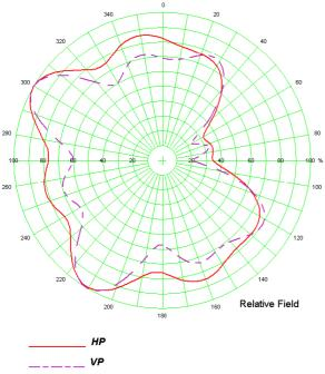
Figure G4: Antenna pattern of antenna A
