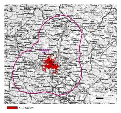
Figure E7: Interference contour of FM transmitter Biebertal 92.6 MHz
