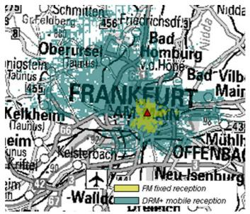
Figure C7: DRM+ mobile (4-QAM 1/3) versus FM fixed reception
