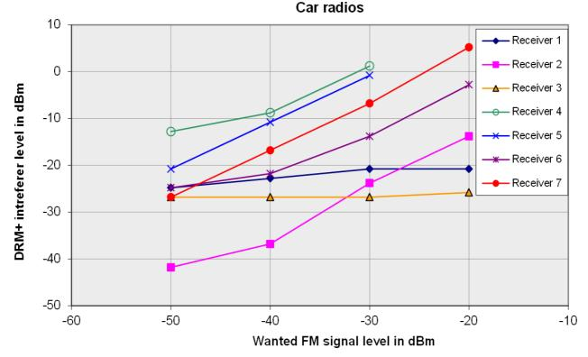
Figure F9: Allowable level of digital interfering signal vs. wanted FM signal level (car receivers)
