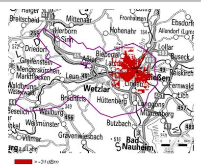
Figure E8: Interference contour of FM transmitter Asslar 93.2 MHz
