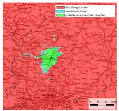
Figure E13: DRM+ portable indoor handheld reception (4-QAM 1/3)
