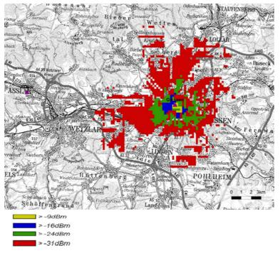
Figure E14: Regions potentially affected by cross-modulation
