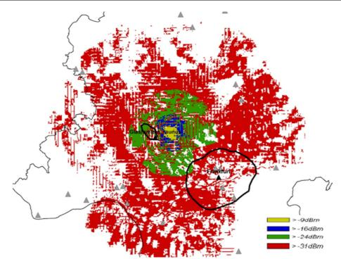
Figure D7: Regions potentially affected by cross-modulation
