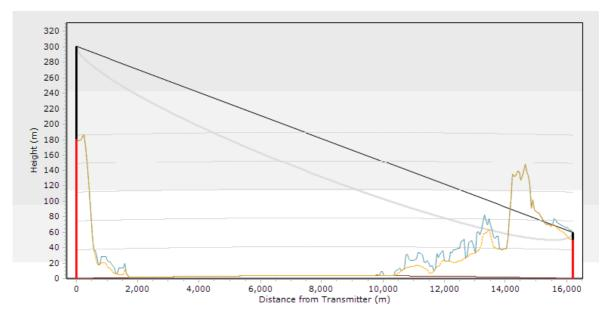
Figure G21: Path profile for dark blue ring in Figure G20
