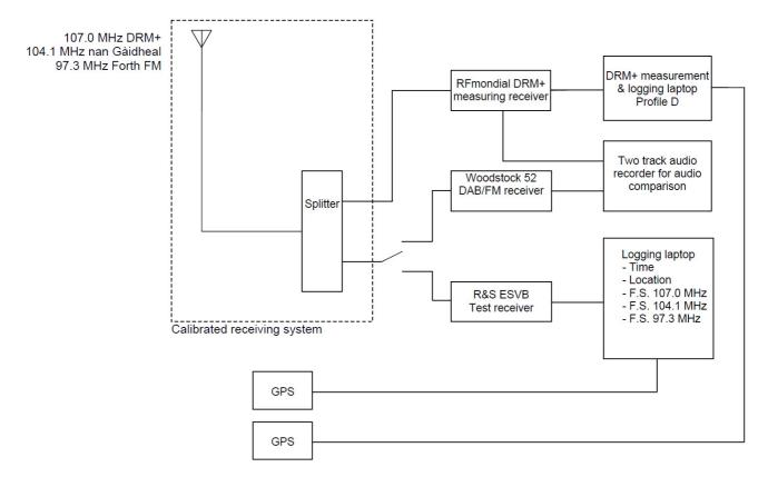
Figure G10: Receiver equipment schematic
