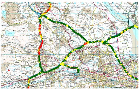
Figure G30: Falkirk to Stirling coverage, 16-QAM, rate 1/2
