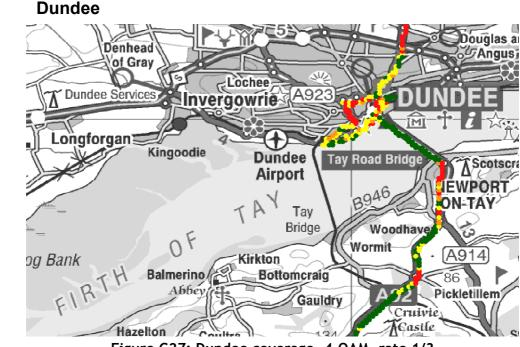
Figure G27: Dundee coverage, 4-QAM, rate 1/3
