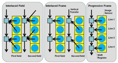
Figure 4: Image sensor readout mode (e.g. CCD)
