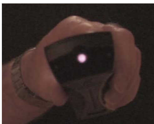
Figure 13: Infra red output of a remote control
