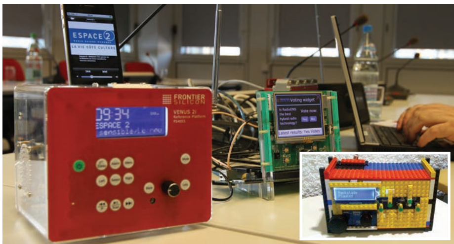
RADIODNS VOTING APPLICATION BASED ON A RECEIVER CHIP FROM FRONTIER SILICON; INSET: LEGO DAB RADIO BUILT USING MXLAB'S DIGITAL RADIO KIT
